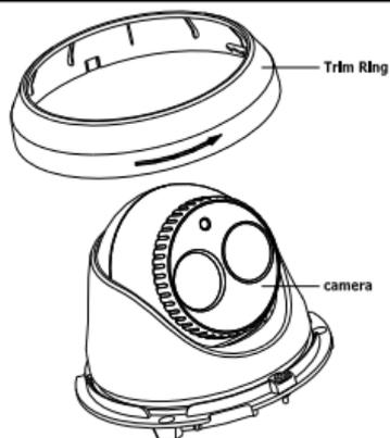
Figure 2-1 Disassembling the Trim Ring
