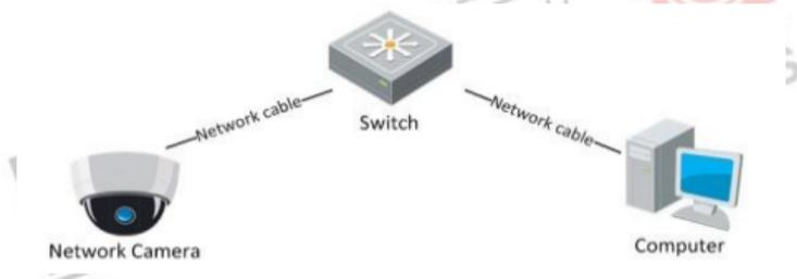
Figure 3-1 Wiring over LAN
