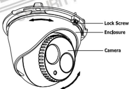
Figure 2-6 Adjust the Lens
