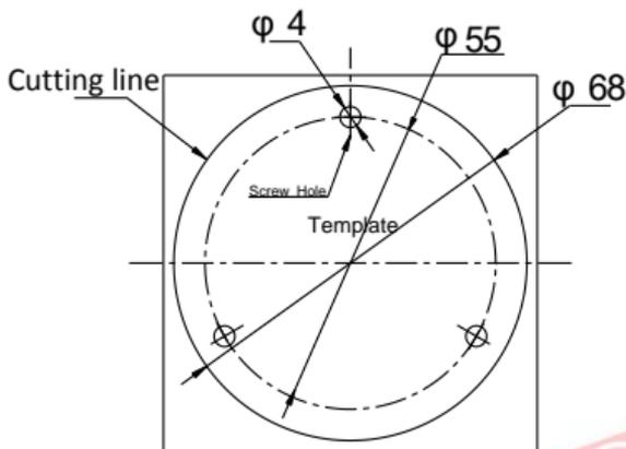
Figure 2-1 Attach the template
