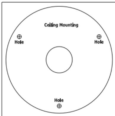
Figure 2-2 The Drill Template
