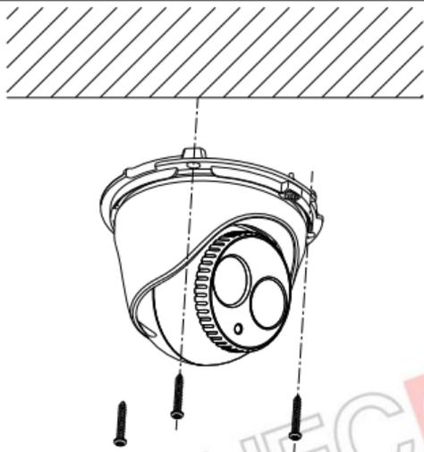
Figure 2-4 Secure the Camera to the Ceiling
