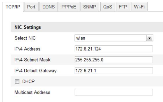
The screenshot shows a web-based configuration interface for TCP/IP settings. At the top, there are several tabs: TCP/IP (selected), Port, DDNS, PPPoE, SNMP, QoS, FTP, and Wi-Fi. Below the tabs is a section titled "NIC Settings". It contains the following fields:
